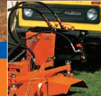
Single-Circuit and Three-Circuit Hydraulics
